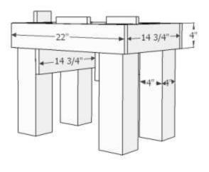
The purpose of the short boards on the inner sides and back of the stand that protrude above the top of the platform are to assist the bottom board in stabilization and prevent it from moving left/right or backwards.
